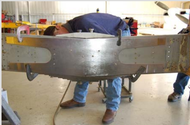
Large Butterfly Doubler Installation
