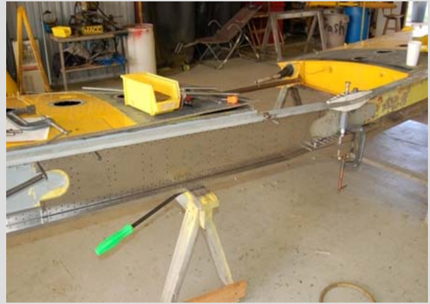
Match Drilling of Spar Doubler
